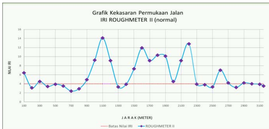
Figure 1. Road surface roughness graph of Alamsyah RPN street from normal direction ( Roughmeter II )
